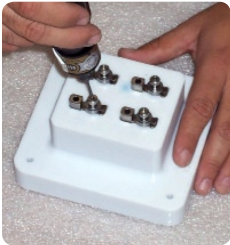
Figure 4: A roller arm fixture assists in assembly. Versus CNC and EDM, there was a 94 percent cost reduction when made with FDM. Cost estimate of part pictured:
