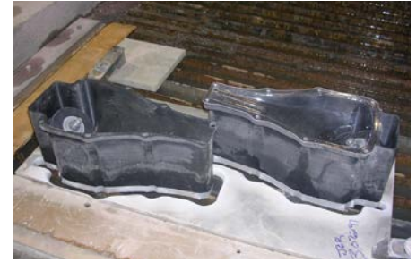
A clear “NACA duct” nests in the pocket of the fixture on the right. The fixture was designed and manufactured in a single day.
