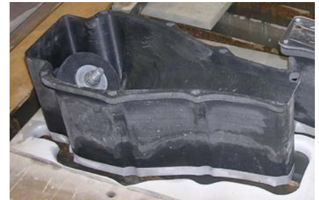
The fixture’s deep pocket would have been difficult to machine, but it was no problem for direct digital manufacturing.
