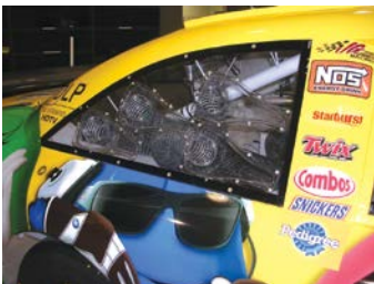
Borrowed from the aerospace industry, NACA ducts draw in air with no appreciable drag. Ducts are shown mounted in the rear window of JGR's #18 M&M car.
