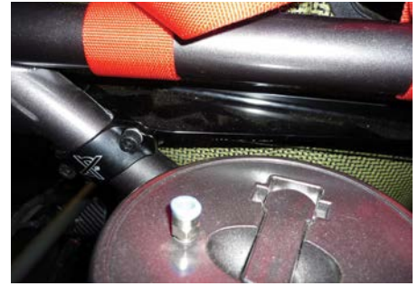
Triple Eight 3D printed the prototype of this seat mount in the racing car.
