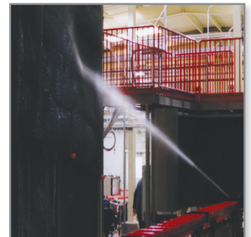
Image 2: Pressure-testing a working prototype at 100 psi
