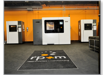
rp+m's hub of innovation located within Thogus Products Company: Two Fortus 400mc machines a Fortus 900mc machine.
