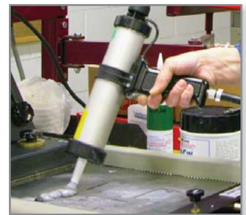
In production, the "goo guns" dispense thermal interface material, which protects electronic components from heat.
