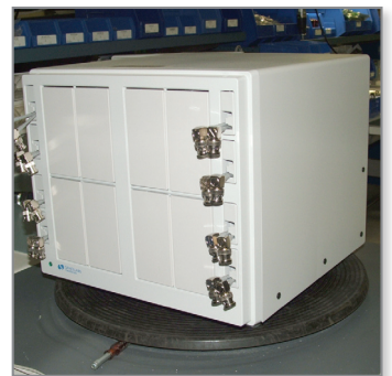
Image 5: Besides securing eight pairs of cables, the snap fit connectors allow these cables to be organized and neat in appearance.
