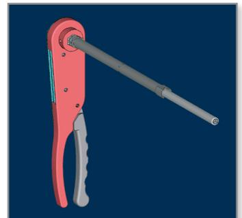
Image 2: ProEngineer was used to design the surgical ratchet.
