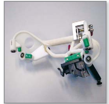
Image 4: Produced with direct digital manufacturing, this tool is used to attach bumper supports.
