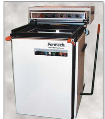
Figure 8: Formech 660 has push-button controls, 24.5x24.5 inch (622x622 mm) forming area and 16 inch (408 mm) draw depth.
