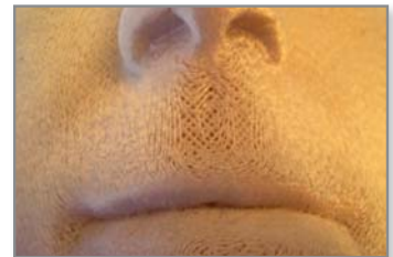
Figure 7: Close up of the tool in figure 6 shows the porosity that results from modified build parameters.
