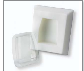
Packaging thermoformed using an FDM mold.
