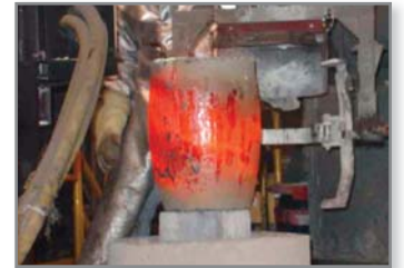
Figure 13: Crucible, filled with molten bronze, just prior to pouring into the mold
