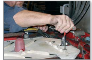
Figure 9: The FDM matchplate is mounted to the automatic molding machine's pattern frame.
