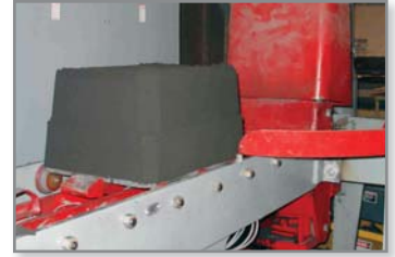
Figure 12: Assembled mold is transferred to the pouring station..
