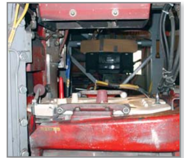
Figure 10: FDM matchplate is raised and mated with the flask for packing the sand casting tool.
