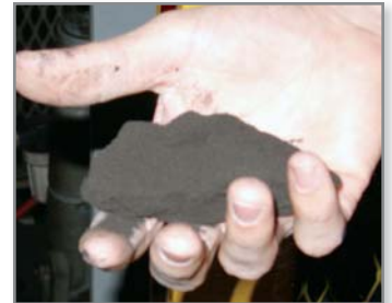
Figure 4: Green sand, as shown here, retains its shape when compacted.
