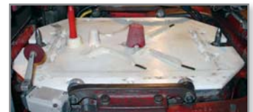
Figure 2: FDM matchplate, mounted in automatic molding machine, can withstand the ramming forces used to pack sand casting tools.
