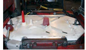
Figure 8: FDM matchplate made in ABS with sprue attached.
