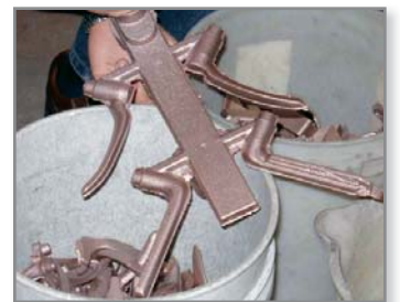
Figure 15: Raw bronze casting, with gates, runner, riser and sprue, is ready for machining.
