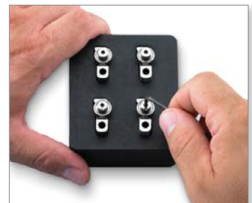
Figure 2: A roller arm fixture assists in assembly. Versus CNC and FDM, there was a 94 percent cost reduction when made with FDM:
