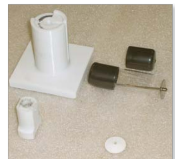
Figure 7: All FDM materials are suitable for manufacturing tools. Pictured is an ABS fixture for mounting a heat shield.
